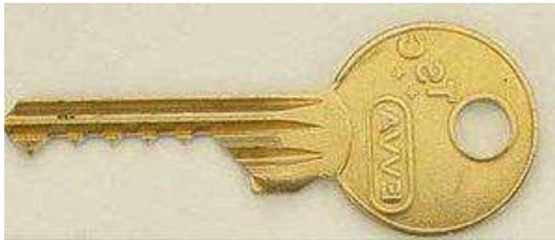
Above: a typical bump key
